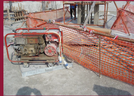
EARTH GROUNDING MUST BE INSTALLED PRIOR TO USE WITH DRIP PAN, FIRE EXTINGUISHER AND PROPER ELECTRICAL PLUG.
