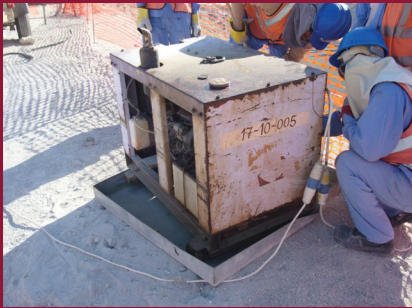
PORTABLE GENERATOR HAS NO EARTHING, NO FIRE EXTINGUISHER
